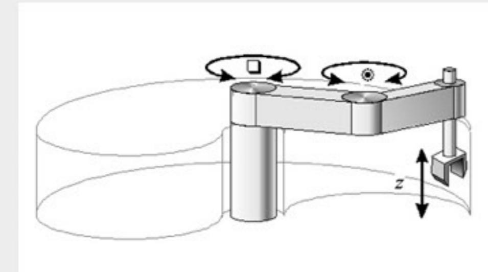
SCARA robots offer a more complete solution than the Cartesian or Cylindrical. It features two parallel joints that provide compliance in one selected plane. They are all-in-one robots, meaning a SCARA robot is equipped with x, y, z and rotary motion (4-axis) in one package that comes ready-to-go, apart from the end-of-arm tooling.
