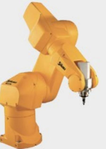
The odds of any of you actually seeing a 5-axis articulated robot will higher than winning the Lottery. Stäubli introduced 5-axis models of their robot intended as a supplement or replacement of expensive 5-axis CNC machines. They created this model by blocking the J6 and replacing it with a machining spindle.
