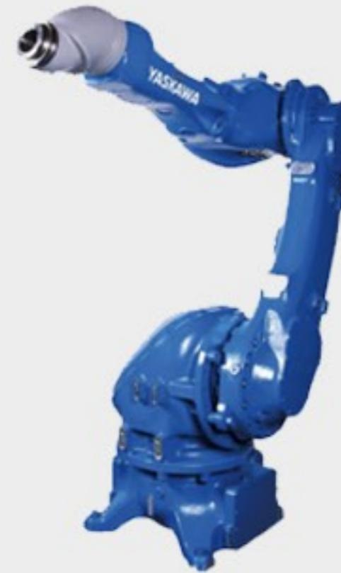
These types of robot are typically found in paint spraying facilities where the robot must be sealed tightly against contamination or to prevent explosions.
