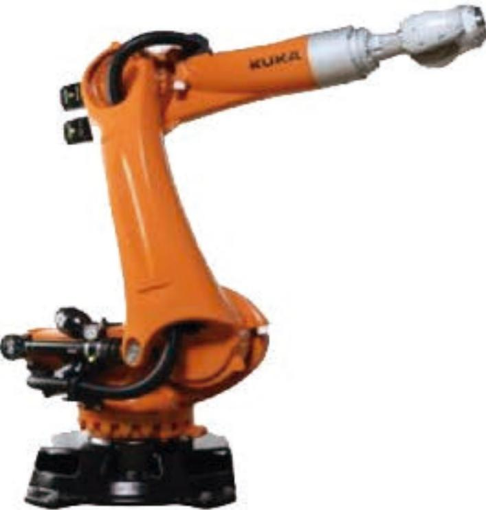
This robot design features rotary joints and can range from simple two joint structures to 10 or more revolute joints. The arm is connected to the base with a twisting joint. The links in the arm are connected by rotary joints. Each joint is called an axis and provides an additional degree of freedom, or range of motion. Industrial robots commonly have four or six electromechanically driven axes.
