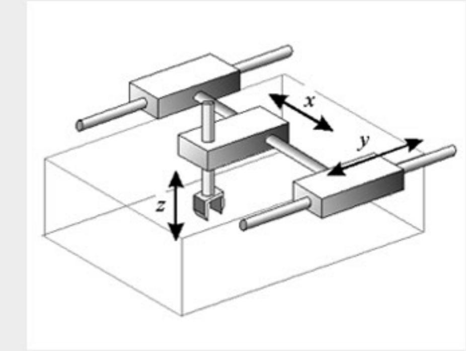
Cartesian robots are also called rectilinear or gantry robots. They are the most common type of robot used in industry. Cartesian robots have three prismatic joints that use the Cartesian coordinate system (X, Y, and Z). They may have an attached wrist to allow for additional rotational movement. The three prismatic joints deliver a linear motion along the axis and the workspace is in the form of a box.
