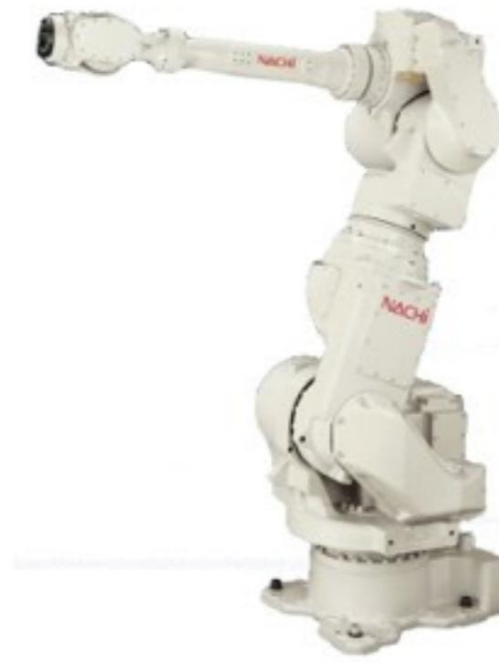
Some robot manufacturers add an additional joint between the 2nd and 3rd axis. The redundant 7-Axis design provides increased freedom of motion and helps achieve optimum robot posture in difficult configurations, especially welding in tight places.
