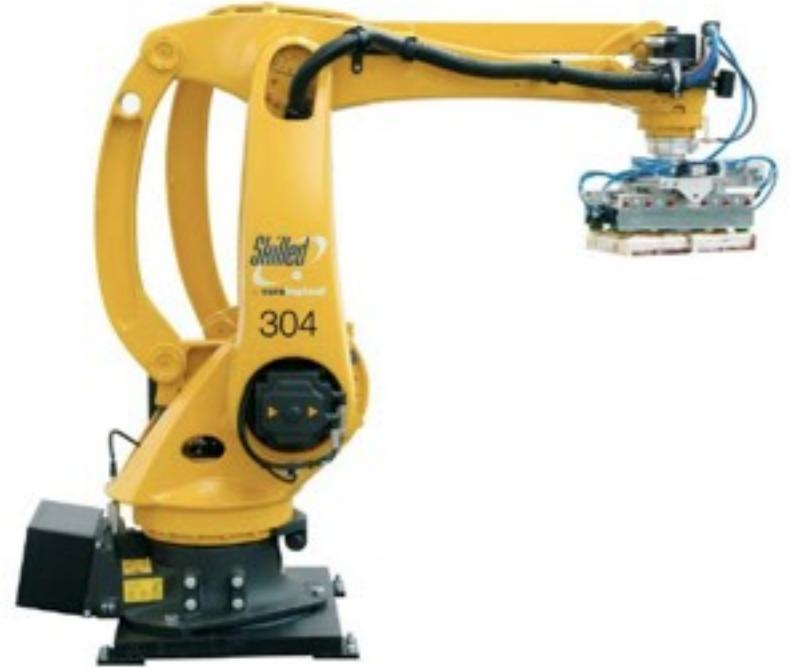
4-axis articulated robots are primarily used for the transfer of materials (pick & place). Notice the link between first joint and the J3 arm. This keep the handling device always parallel with the base (floor) plate.
