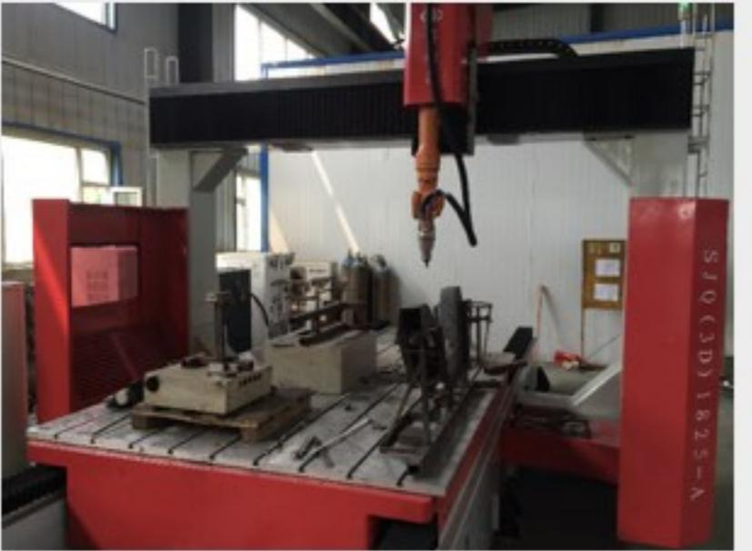
Kuka-China has developed an interesting hybrid robot that combines the versatility of a robot wrist and the accuracy and large workspace of a gantry cartesian robot.
