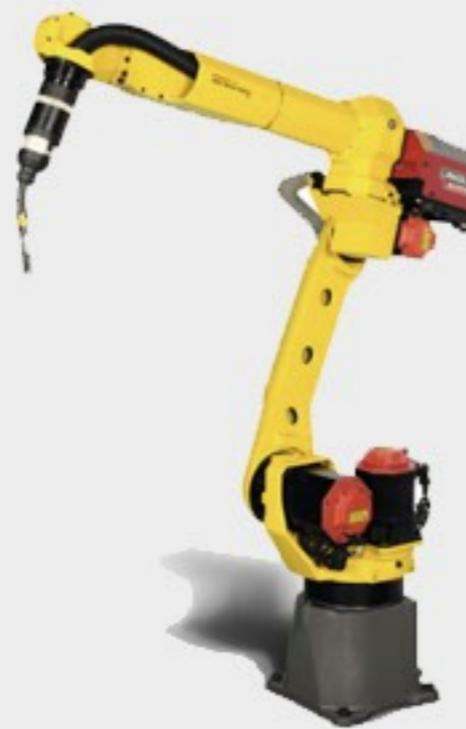
An offset wrist and/or offset joint robot has the centerline of the wrist offset from the centerline of the adjacent axis. The offset wrist design is typically used for welding since it allows the placement of a through-arm design.
