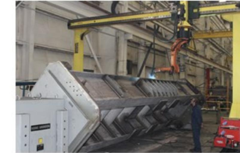
A few large part welding shops will even combine a single horizontal axis or a 2-axis rotary table with a 3-axis gantry. This combination gives the production team the possibility to complete a wide range of complex parts.
