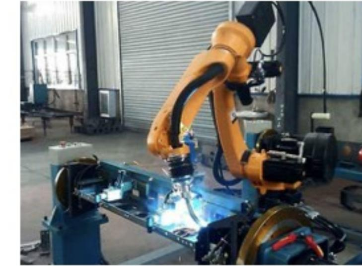
Rotary tables come in many forms, configuration and sizes. They can be 1-axis, 2-axis, vertical, horizontal or even mounted on a single axis horizontal positioner. The motion of the rotary tables can be indexed (stationary while welding) or synchronous (rotating while the welding) if they have the correct motors and the control capability. For large object welding there are robust 2-axis rotary tables mounted on arm that be positioned vertically.
