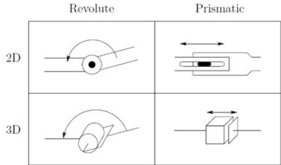
Before we present the different types of robots we must first introduce the concept of "degree of freedom" which is also known as an axis. An axis is a point of rotational (Revolute) or the line of linear movement (Prismatic). For example, a typical CNC milling machine has 3 prismatic axes and industrial robots typically have 6 revolute axes of rotation.
