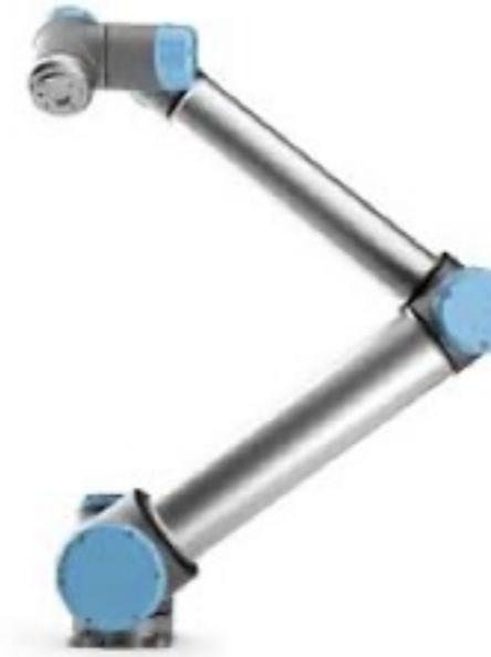
This type of 6-axis articulated robot has each axis offset from the adjacent axis. The smaller drive motors are in the interior of the arm/joint. The offset joint robots are widely used in machine loading tasks due to their lower costs, ease of teaching and the integrated torque control sensor on each axis. This configuration will stop the robot movement if it collides with an object or more importantly, a person.
