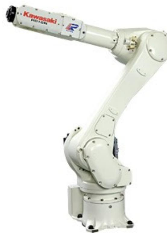
The most popular and versatile industrial robot used in manufacturing is the 6-axis articulated spherical joint robot.
