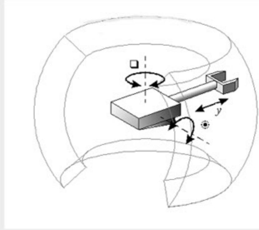
Spherical robots, also known as polar robots, are like cylindrical robots, but instead of having one rotary joint and two linear joints, they have two rotary joints and one linear joint. These robots can be used in some of the most basic robotic such as painting, welding, and assembly.
