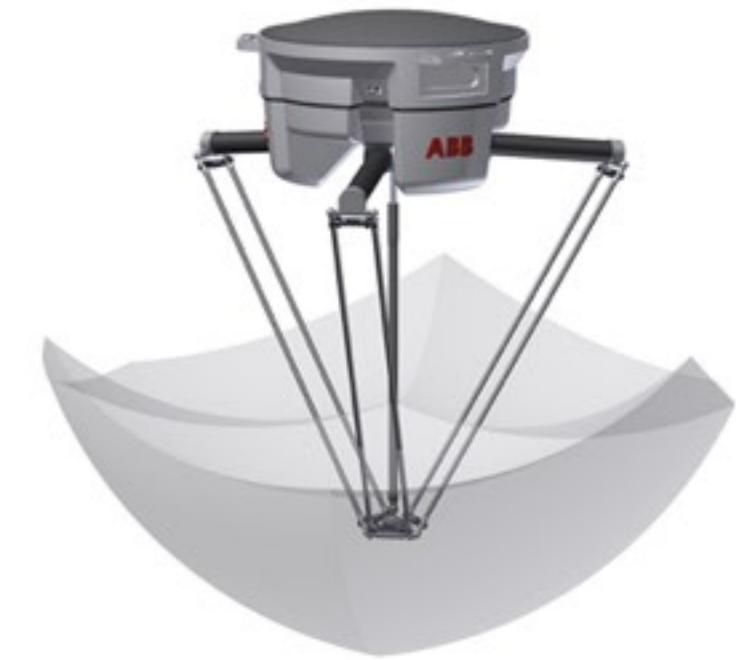
Delta robots are the fastest and often most expensive. These spider-like robots are built from jointed parallelograms connected to a common base. They have a unique, truncated sphere work envelop and their main advantage is their speed and precision with which they operate.
