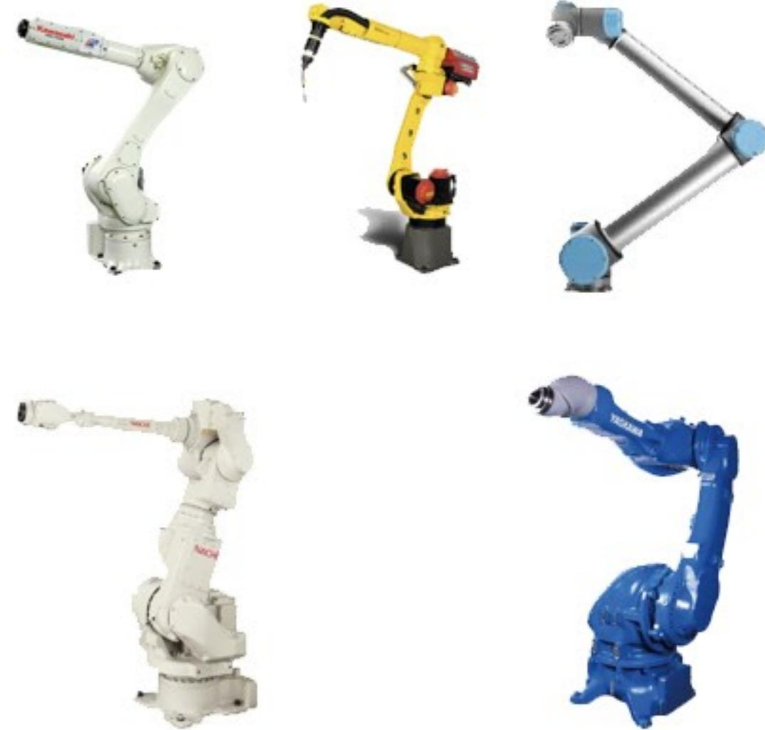
There are sub-group types of 6-axis articulated robots with differing joint methods design for specific processes or markets.
