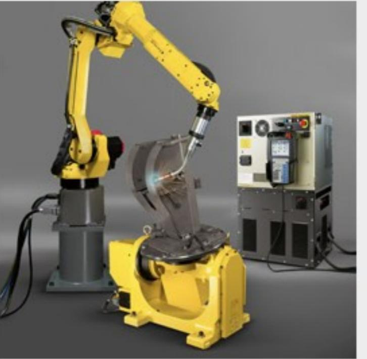
A 6-axis robot can be assembled with a single rotary table or a 2-axis combination table as pictured. A rotary table allows the production team to rotate the part while keeping an optimal robot configuration.
