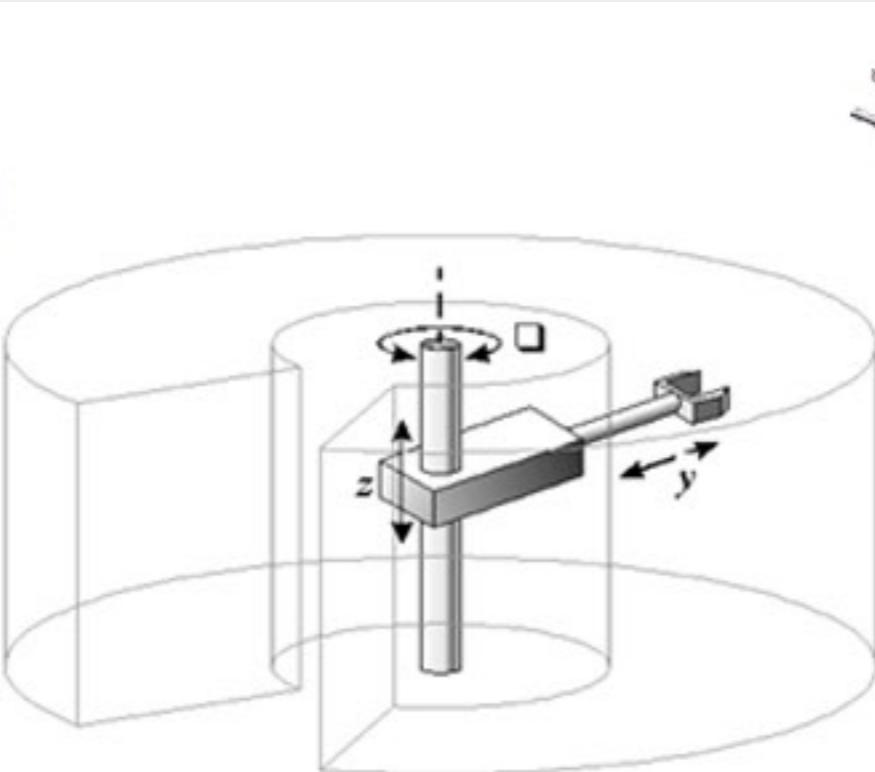
Cylindrical robots are very simple and like Cartesian in their axis of motion. Most Cylindrical robots are made of two moving elements: rotary and linear actuators. Because they have a cylindrical work envelope, machine designers might select them for their economy of space.
