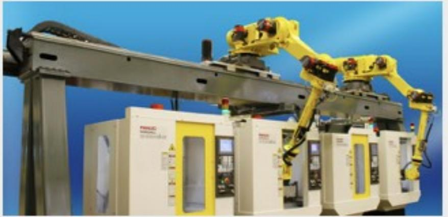
6-axis robots can be attached to linear axis rails to extend the robot's workspace envelop. A robot mounted on a single linear axis provides the advantage of working on long objects or workspaces while keeping the robot in an optimal configuration. The rails can range from 2m to 30m or more.
